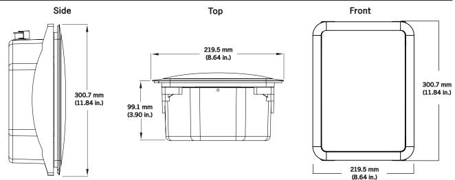
**Optional Accessories - Pre-Construction Bracket (AC-IW5-PCB)**
