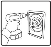
**6.** Remove paint mask. Then tighten the four clamping screws. DO NOT OVER TIGHTEN.
