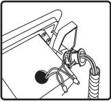
**4.** Connect speaker wires to wire leads using wirenuts. Push wire nuts into backcan and insert conduit clamp.
