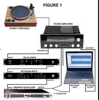
The labeling of many panel and input/output connectors used on amplifiers and recorders can be be quite different. So, connections may vary. Last resort: Use an outboard preamp with the *RE-EQUALIZER III*, and feed an unused AUX input on your amplifier.
