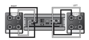
Most of the audio signal going to the speakers drives the bass units. Where one cable feeds both bass and treble units, this heavy bass current can modulate the high frequencies. Using separate cables for treble and bass units reduces intermodulation effects and improves headroom and clarity. This technique of wiring is known as Bi-Wiring. To bi-wire, you will need to install two lengths of twin core cable between the amplifier and each loudspeaker.
