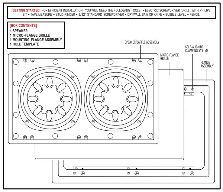
Thank you for purchasing the Phase Technology<sup>®</sup> IW-210 high definition in-wall subwoofer. The mounting frame of extruded aluminum has a uniquely designed self-aligning clamping system to secure the flange assembly to the drywall. This patented design simplifies installation and reduces unwanted wall vibration resulting in improved performance and definition. The IW-210 is a passive subwoofer and is designed to be used with the Phase Technology P350 subwoofer amplifier.
