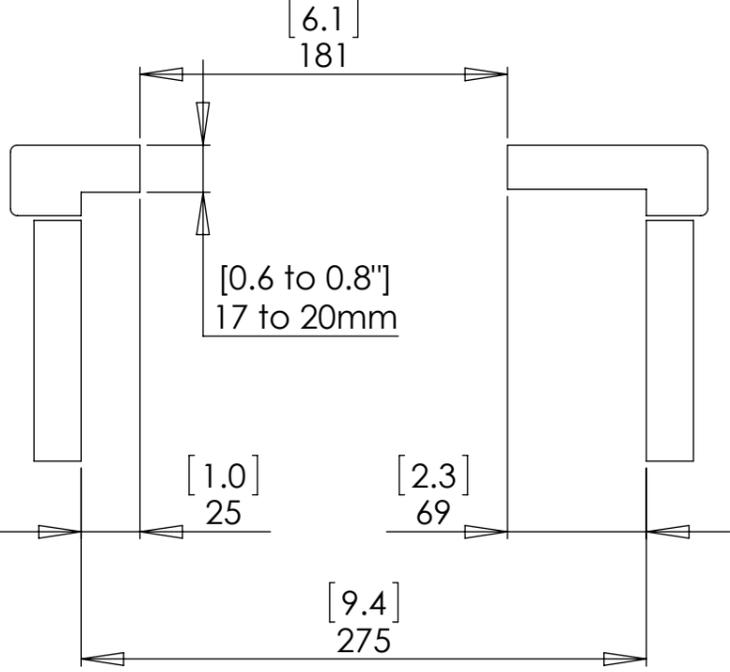
The section above shows the use of a thicker cabinet top. This is possible but the top thickness around the mechanism must be between 17 and 20mm.
