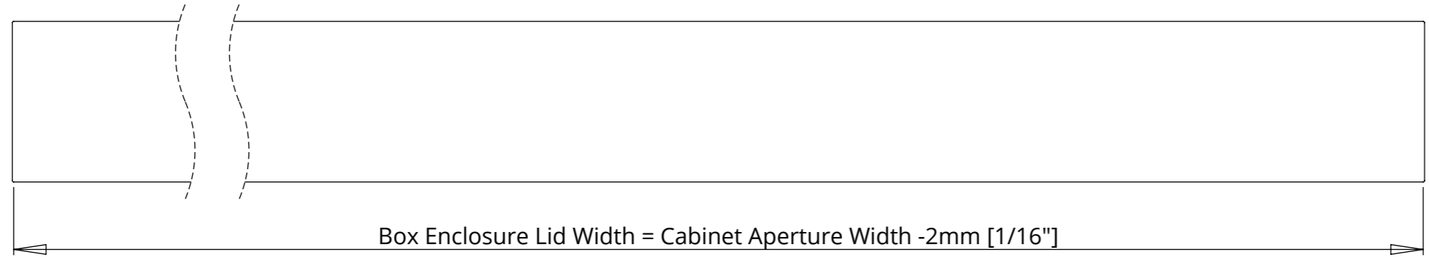
BOX ENCLOSURE LID (TAPERED) TOP VIEW
