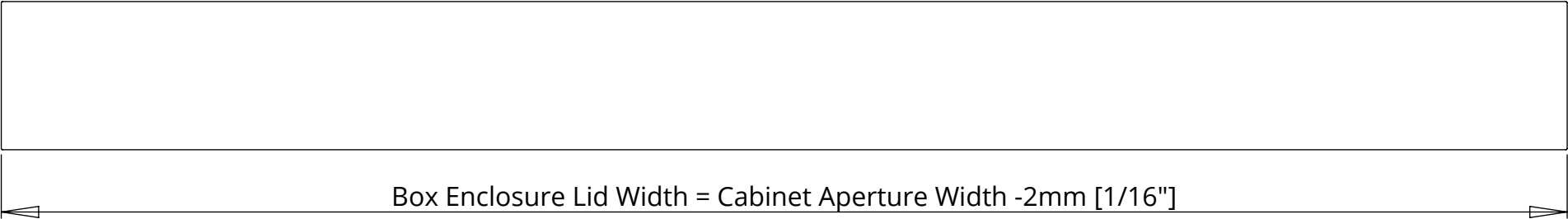
BOX ENCLOSURE LID (TAPERED) - TOP VIEW
