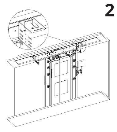
Fix the Base Panel onto the Base Panel Brackets from underneath
