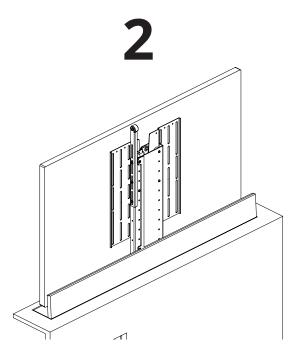
Once the screen is at the desired height, adjust the Push Roller so that the top of it sits approximately 5mm [0.2"] above the top of the screen  The height of the screen can be adjusted by removing the screen and changing the height of the four toggles that the KH Mount Plate hooks on to.
