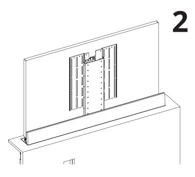
The height of the screen can be adjusted by removing the screen and changing the height of the four toggles that the KH Mount Plate hooks on to.
