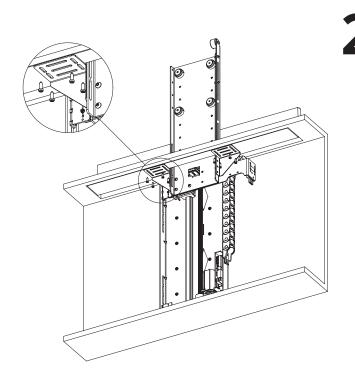
Fix the Base Panel onto the Base Panel Brackets from underneath
