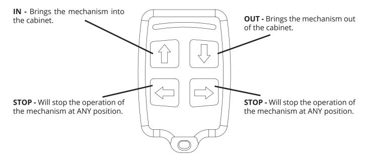
The Radio Frequency (RF) Remote Control can only be used to recall the above functions.
