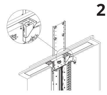
Fix the Base Panel onto the Base Panel Brackets from underneath
