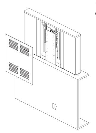
Place the rear of the Box Enclosure onto the lift and secure in place at the sides.
