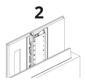
The height of the screen can be adjusted by removing the screen and changing the height of the four toggles that the KH Mount Plate hooks on to.
