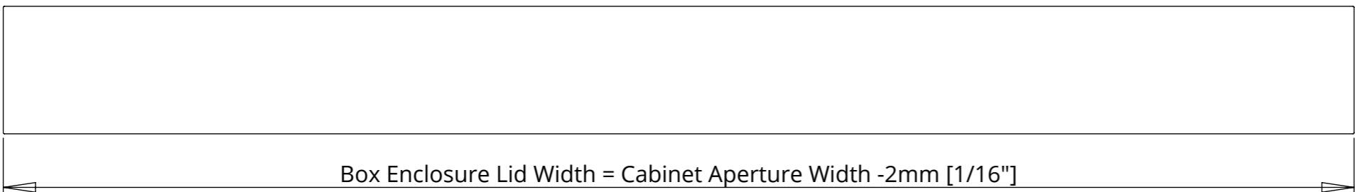
BOX ENCLOSURE LID (TAPERED) - TOP VIEW
