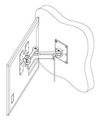
Run cables to the back of the TV and secure in place using the provide cable management hook.
