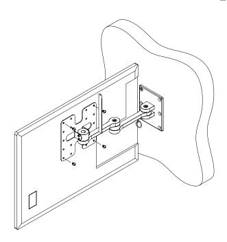
Fully extend the bracket and turn the FSA2 screen mount to 90° for better access. Hold the screen up to the FSA2 screen mount and fix in place using suitable fixings from the provided fixings pack.
