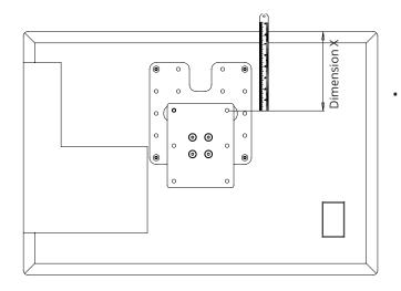
Measure from the top of the screen, down to the top mounting hole on the Wall Plate (Dimension X) to determine positioning of the top wall fixing holes.
