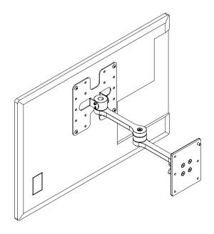
Place the FSA2 on the back of the screen, lining up the mount holes in the FSA2 Screen Plate with the VESA mount holes in the back of the TV.
