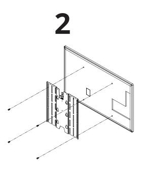
With the screen attached, the mount plate can be hooked onto the corresponding mount boss, and secured in place by rotating the locking lever 90°.
