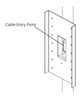
All cables can be easily routed behind the screen through the cable entry point
