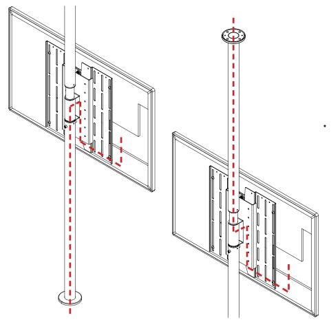
Cables can be routed down through the FCM Bottom Tube and into the floor, or up through the FCM Top Tube and into the ceiling.
