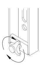
To help levelling, the screen can be tilted forwards or backwards slightly by winding the two Levelling Wheels in or out at the bottom of the Screen Uprights.
