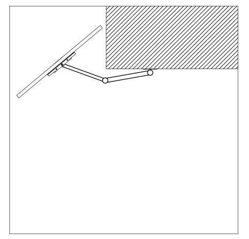
To store the screen facing one direction and still be able to move the screen up to 180 around a corner to another viewing area. To fix the screen to one wall of a room corner installation.
