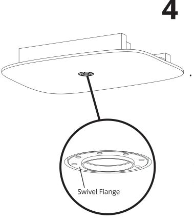
With all mounting options the Swivel Flange should sit flush with the ceieling
