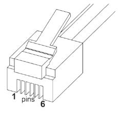
SERIAL PIN LAYOUT PIN 2: RX PIN 3: TX PIN 5: GROUND
