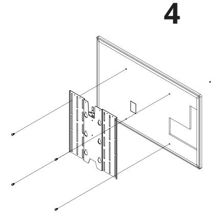
Secure the screen mount to the mount holes on the back of the screen using the bolts provided.
