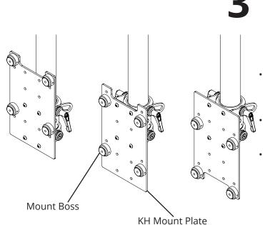
Screen Mount height can be adjusted by using the higher or lower fixing holes in the middle of the KH Mount Plate.
