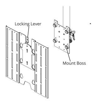
With the screen attached, the mount plate can be hooked onto the corresponding mount boss, and secured in place by rotating the locking lever 90°.
