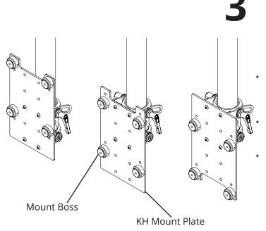
Screen Mount height can be adjusted by using the higher or lower fixing holes in the middle of the KH Mount Plate.
