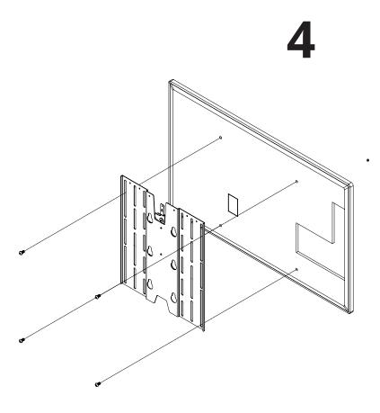
Secure the screen mount to the mount holes on the back of the screen using the bolts provided.
