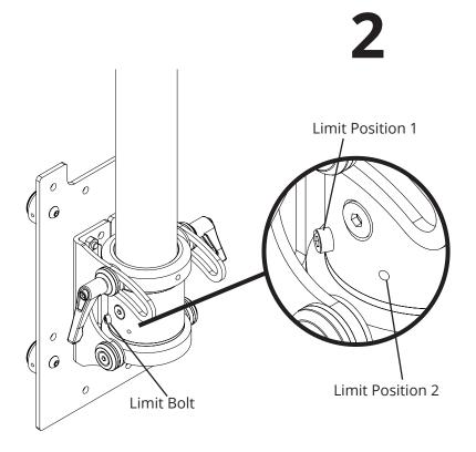
Two M6 cap headbolts are provided to limit the rotation of the FM. Locate them in the desired location to limit rotation as required.
