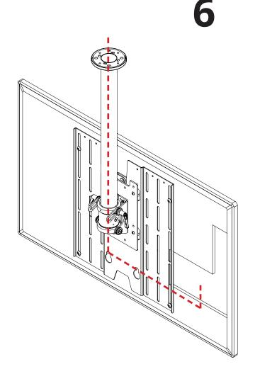
Cables can be routed up through the CM Pole and into the ceiling.
