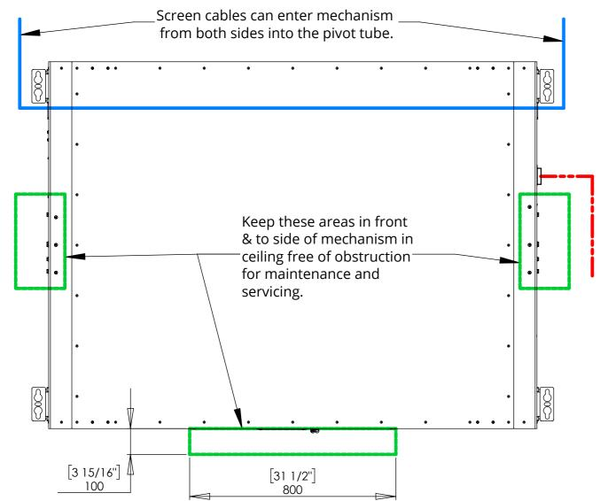
Cables for the screen can be routed in from both sides, allowing for power and signal cables to be separated when entering the mechanism.
