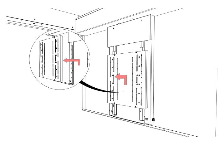
Once unlocked, the mount plate will lift up approximatley 20mm [0.8"] and can be pulled forward away from the hinging tray.
