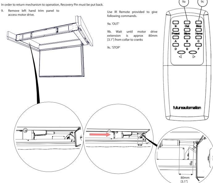
To return the Recovery Pin, manually lift the hinging tray back towards CLOSED position.
