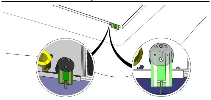
Esnure card is securley inserted into override connector. Card should click into position and be held in position by the connector.
