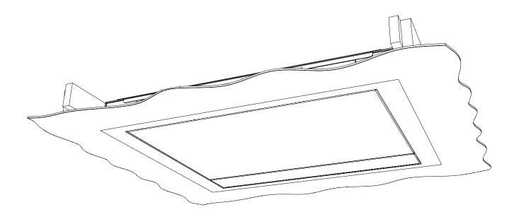
With MDF Plaster Trims secured in place the ceiling can be fitted around the mechansim and plastered.
