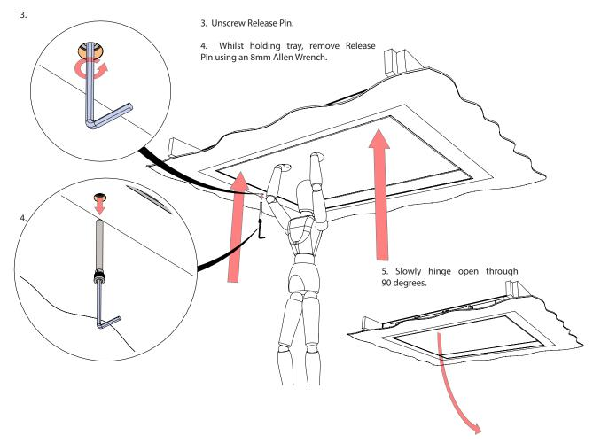
**Accessing Control Board and Connections**
