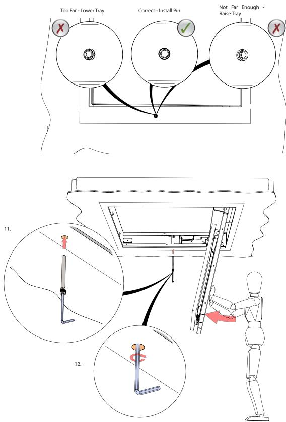
With pin in place, carefully operate the mechanism via the IR Remote.
