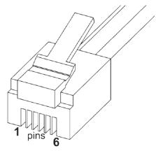
Serial Pin Layout PIN 2: RX PIN 3: TX PIN 5: GROUND
