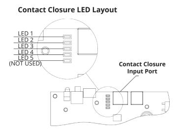
NOTE: A short on any pin while the mechanism is operating will execute a STOP command and disable Contact Closure input for 1 second.
