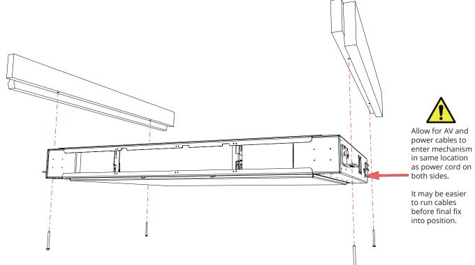
Mechanism mount plates allow up to 12mm [0.5"] diameter fixings to be
