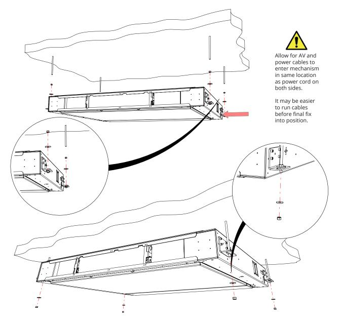
To hang mechanism on studs fixed securely to the ceiling above, suitable fixings should be used (Not Provided).
