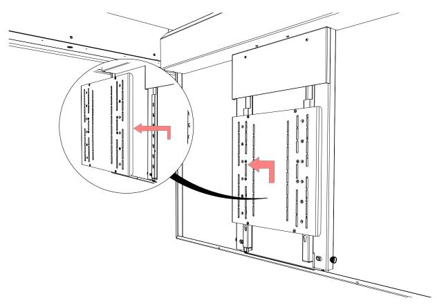
Once unlocked, the mount plate will lift up approximately 20mm [0.8"] and can be pulled forward away from the hinging tray. Cables can now be routed through the mechanism.
