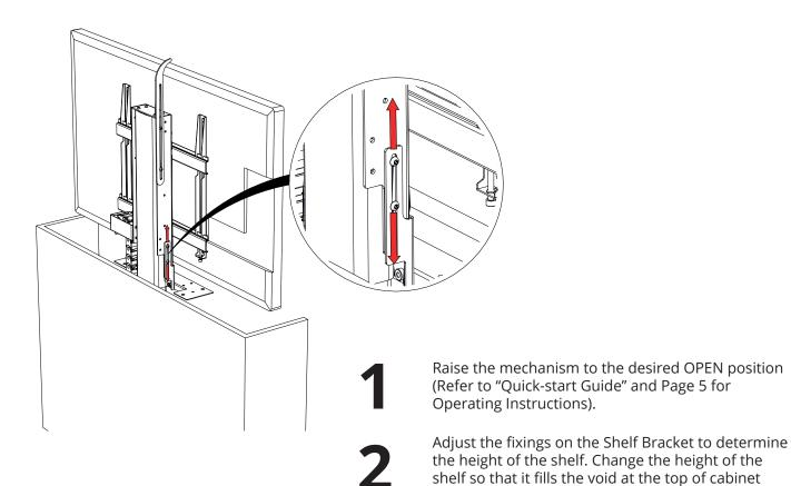
Slide the shelf material into place under the screen on top of the Base Shelf.
