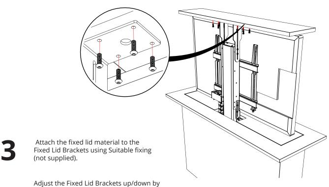
loosening the 2 bolts securing each bracket an sliding the fixed lid up/down until it sits level with the surrounding joinery when the mechanism is in the fully CLOSED position.
