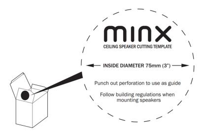
2. When mounting speakers flush to a ceiling or wall, ensure that there is enough depth/clearance within the respective cavity. For the Minx C46 you will require a minimum clearance of **95mm (3** ¾").
