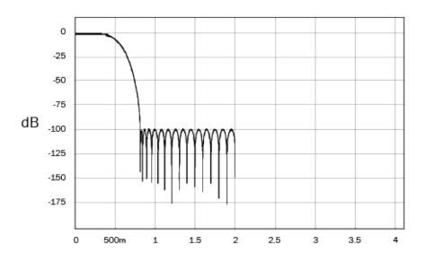
Our Slow filter has a linear phase and is a compromise between some very high frequency roll off and the minimized level of pre/post impulse ringing. Stop band attenuation is less than other filter types, but there's no phase shift and the impulse response is the cleanest.
