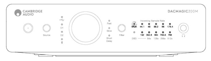
Master Quality Authenticated is an audio codec using a sophisticated compression algorithm, and a form of file authentication intended for highquality audio streaming and file download. This allows the listener to receive digital audio at the original studio quality.
