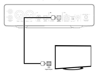
**Important Note:** Only connect one co-axial OR optical cable to each digital input. The unit will not operate properly if both connections are made (even if only one is active).
