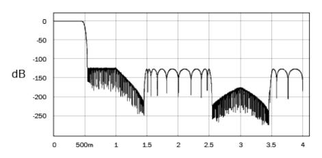
The Fast (Linear Phase) filter is a highly regarded audio filter offering low ripple in both the pass and stop bands, and what is known as constant group delay. Constant group delay means that audio signals of all frequencies are always delayed by the same amount when passing through the filter. All audio is therefore fully time-coherent at the output.
