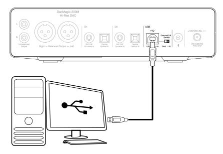
The DacMagic 200M only supports USB audio playback using USB Class 2.0 Audio. For this it is required that the DacMagic 200M is connected to a USB 2.0 port using a suitable USB cable, and we would recommend any USB certified high-speed USB 2.0 'A–B' cable.
