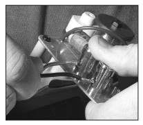
Strip about 1/2" (13 mm) of insulation from the connecting wires. Connect them to the appropriate push terminal, being careful to observe polarity (positive to the red terminal, negative to the black terminal).
