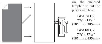
WARNING: Exercise extreme care before making any wall cuts to ensure that you will not cut through any wires, pipes, or other items that may be in the wall. You may sometimes, but not always, be able to determine the approximate location of wires and pipes by looking at the locations of nearby outlets and plumbing. But their location or absence is never an assurance that there is not something within the wall cavity.
