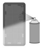
The grille can be painted to blend into virtually any décor. The grille has a removable scrim behind the metal to conceal the drivers. Before painting remove the grille, carefully remove the fabric scrim from the inside of the metal grille using a tweezers or needle-nosed pliers, starting at a corner of the grille and care-
