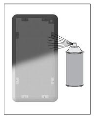
The white plastic frame and the metal grille may be left as is, or painted to match your décor. You can paint the frame before or after it is installed in the wall. Spray painting (using slightly thinned paint) is the best method to use for painting the grille. **Before painting, carefully peel off the scrim cloth from inside the grille.** After painting the grille, use air pressure to "blow out" any grille holes that are filled in with paint, then carefully replace the scrimcloth.
