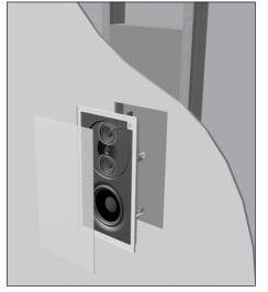
30LCR Back Box. The Back Box provides the correct acoustic environment for the 30 LCR speaker and it is the only way to guarantee that the speaker achieves its THX-certified performance. The rotator clamps (sometimes called "dog legs") will easily grab the combined thickness of 5/8" sheetrock and the 3/8" back box's front panel. The sheetrock must be
