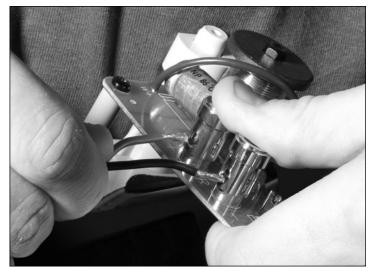
Strip about <sup>1</sup>/<sub>2</sub>" (13 mm) of insulation from the connecting wires. Connect them to the appropriate push terminal, being careful to observe polarity (positive to the red terminal, negative to the black terminal).
