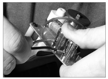
Strip about  $\frac{1}{2}$ " (13 mm) of insulation from the connecting wires. Connect them to the appropriate push terminal, being careful to observe polarity (positive to the red terminal, negative to the black terminal).
