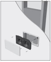
Back Box IN-BOX-155. The Back Box provides the correct acoustic environment for the 155 LCR and ensures its THX-level performance. The rotator clamps (sometimes called "dog legs") will easily grab the combined thickness of 5/8" sheetrock and the 3/8" back box's front panel. The sheetrock must be adhered to the front panel of the back box very solidly and positively. Use very liberal amounts of a high-quality construction adhesive,
