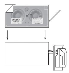
After determining the best location for the speaker as outlined above, use the enclosed template to cut the proper size hole.
