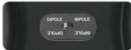
If you are planning to use the IW-155SR in a 5.1, 7.1 or 9.1 Dolby True HD or DTS Master Audio-based home theater, we recommend setting the switch to Dipole mode. Dipole puts the two driver arrays out of acoustic and electric phase with each other, so in the
