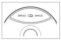
In Dipole mode the 8200e SR and 4200e SR produces ambience with minimal localization (best for most movies and video soundtracks) and more localizable sound in the Bipole mode (preferred for some music recordings). Switching
