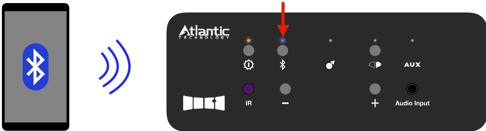
Enter pairing mode on the Bluetooth device you want to connect to the STA-200 and select the STA-200 from the discoverable devices list.
