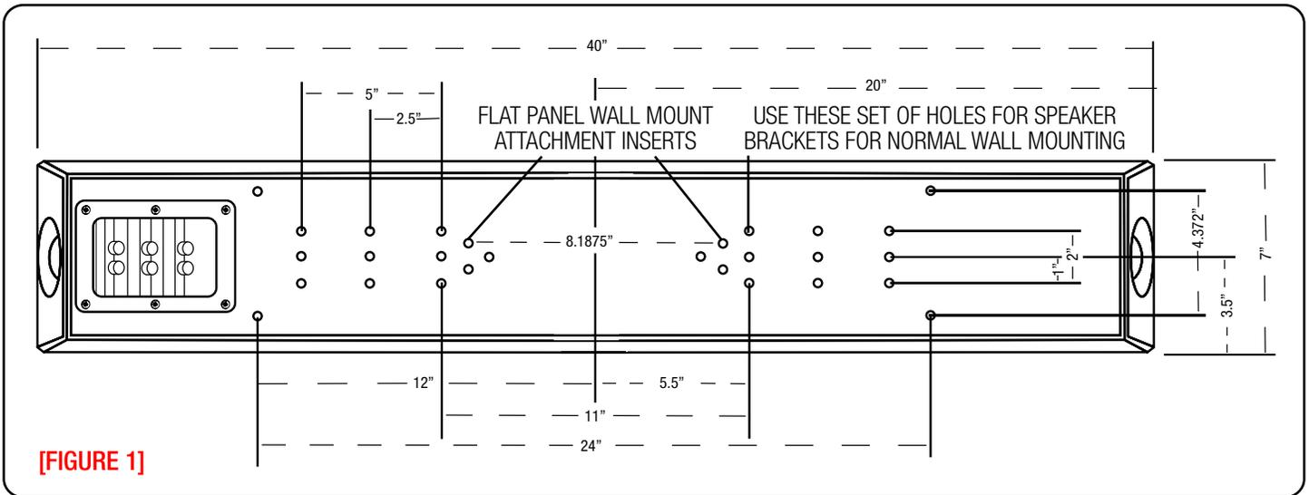
the brackets allow them to be positioned for attaching to 16" on center studs. There are four identical brackets supplied with the speaker. Two are mounted to the wall, two are mounted to the rear of the speaker cabinet.
