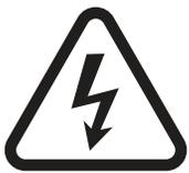
The lightning flash with arrowhead symbol, within an equilateral triangle, is intended to alert you to the presence of un-insulated dangerous voltage within the product's enclosure that may be of sufficient magnitude to constitute a risk of electric shock to persons.
