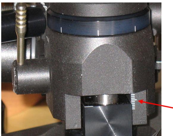
Fig. 2.VTA tower side-rough scale
