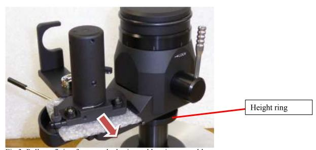
Fig.3. Pull out fixing foam on the horizontal bearing assembly
