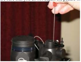
Fig.12. Fixing vertical damping holder
