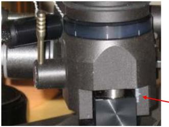
Fig. 10. VTA tower side-rough scale
