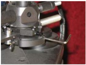
Fig.14 Removing horizontal trough
