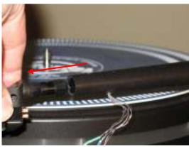
Fig.7B Removing headshell
