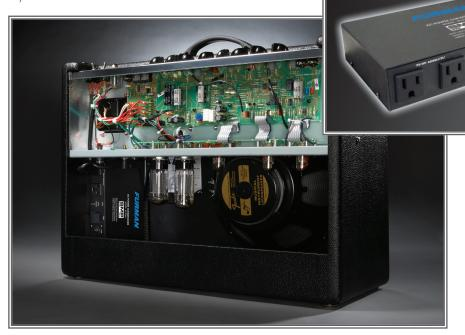
AC-215A mounted inside a guitar amplifier (left) and behind a flat-screen television (above). The slim, compact design is sleek and unobtrusive, allowing for ease of use and discreet mounting anywhere that clean, filtered power is needed.
