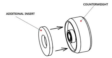
The first part is the counterweight itself. The second part is an additional insert that enables optimal balancing of heavier cartridges.
