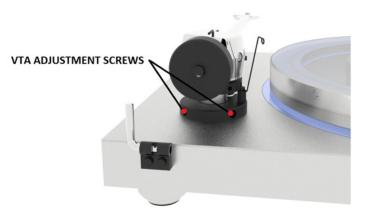
To set the **Vertical Tracking Angle (VTA)**, first put a record (VTF) on the platter. When the needle is lowered into the record groove, the tube of the tonearm should be parallel to the surface of the record. If it is not, loosen both hexagonal screws in the tonearm base, just enough to allow vertical movement of the arm pillar without force, and slide the arm up or down until it is parallel.
