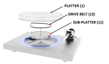
Remove the protective cover from the sub-platter (11). Install the sub-platter (11), drive belt (12) and platter (1) as shown in the above illustration.
