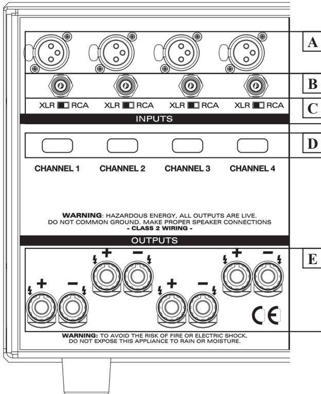
Above shows channel section 1-4. Channel section 5-8 is a mirror image. See Appendix F for complete view.
